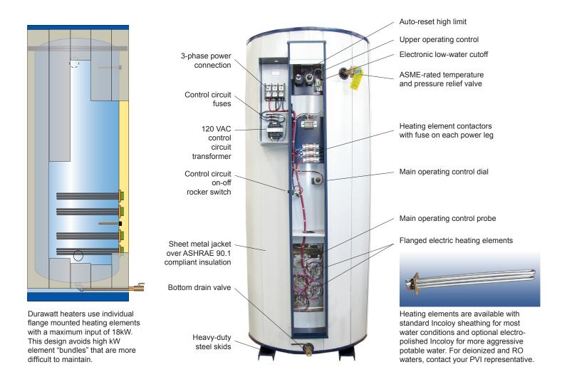
Typical construction shown with standard equipment.
