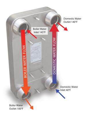
Inside the plate exchanger, counter-flows of boiler and domestic water maximize the temperature differentials and allow the temperatures of the opposing liquids to "cross" with boiler return water becoming colder than domestic outlet water.
