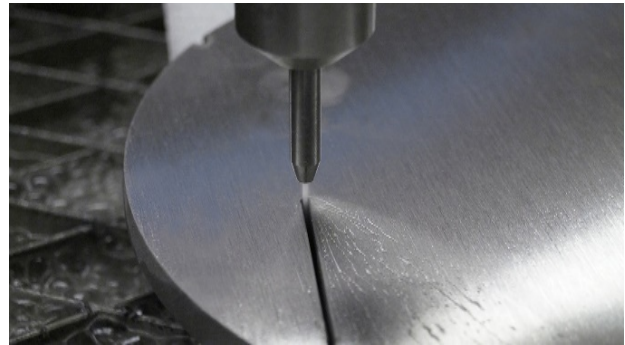
Figure 1: 50,000 psi Water Jet Cutting with no heat signature
