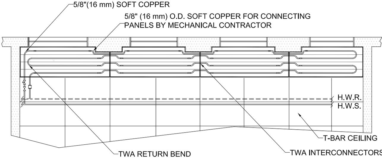
TWA RADIANT PANELS NOTCHED AROUND PERIMETER COLUMNS. EVEN PASS COILING SHOWN
