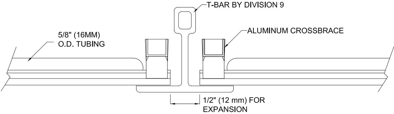
EXPANSION GAP FOR TWA RADIANT PANEL
