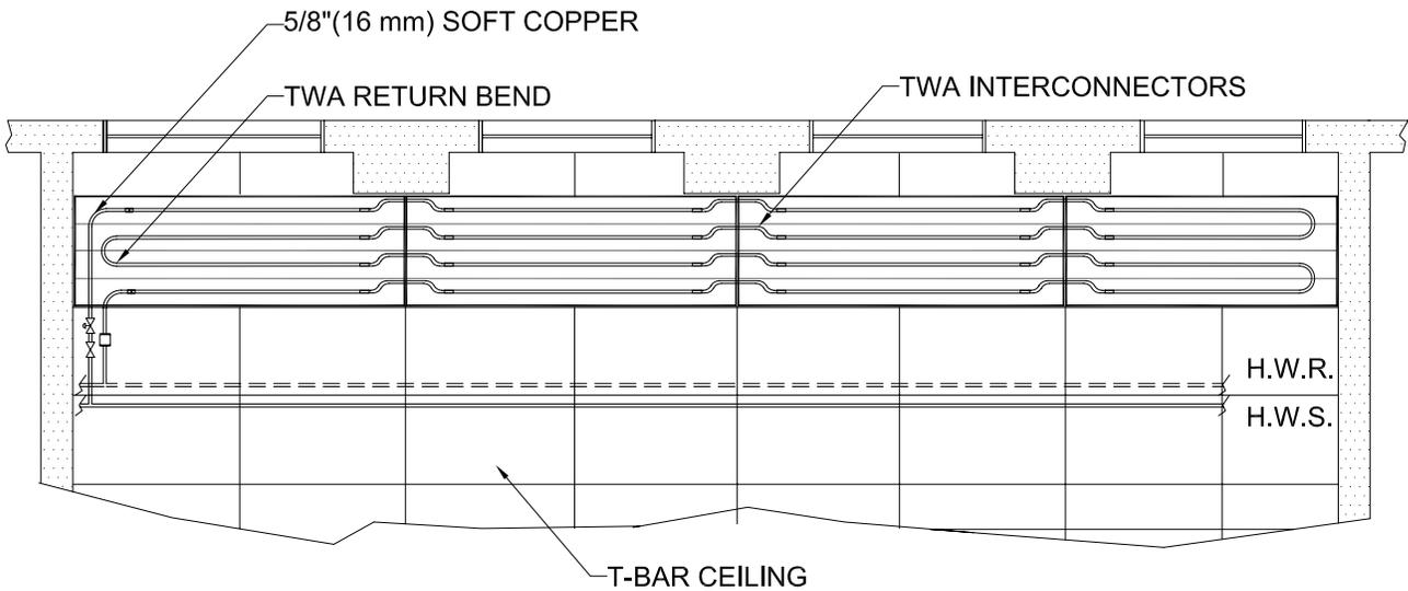
TWA RADIANT PANELS POSITIONED CLEAR OF PERIMETER COLUMNS. EVEN PASS COILING SHOWN
