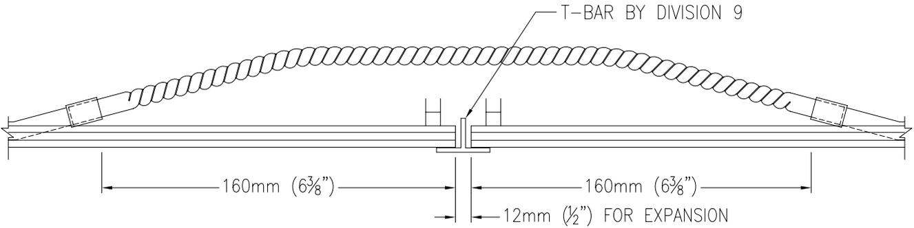
INTERCONNECTORS SUPPLIED BY TWA WHEN PANELS ARE INSTALLED IN SERIES IN THE SAME ROOM
