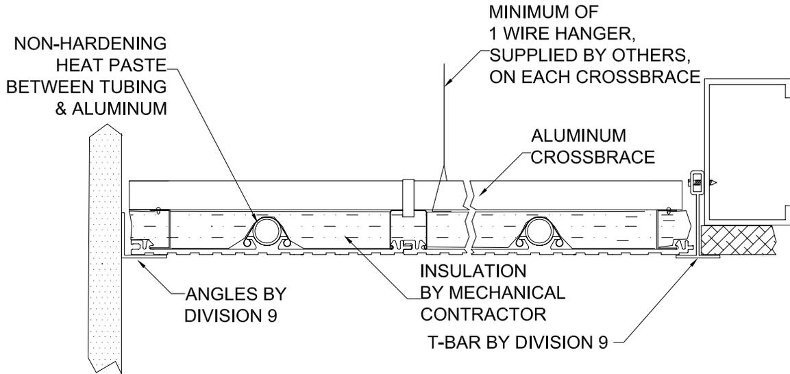
NOTE: OPENING FOR RADIANT PANEL OBTAINED FROM L-7. ACCESS TO SUPPLY, RETURN AND INTERCONNECTION BETWEEN PANELS WILL BE REQUIRED.
