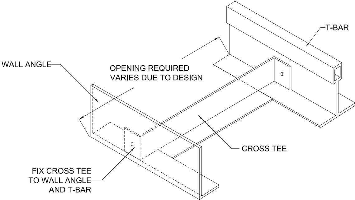
INSTALLATION OF CROSS TEE BETWEEN PANEL ENDS
