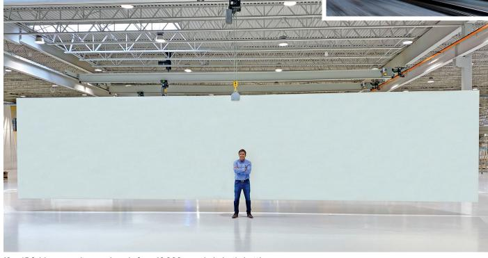
$12 \times 45$  ft biocomposite panel made from 16,000 recycled plastic bottles
