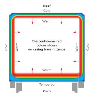
Thermography view of our biocomposite casing: Rooftop example in a winter simulation
