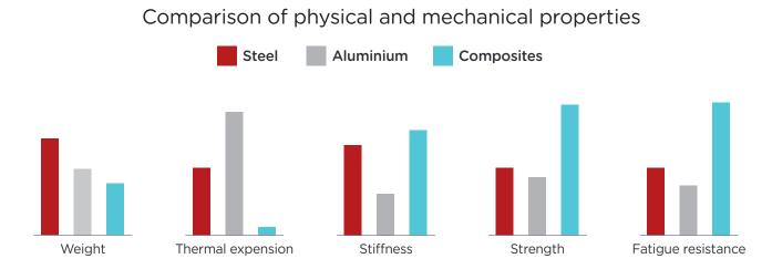
The illustration above compares the physical and mechanical properties of steel, aluminum and composites. As shown, using composites provides more benefits than the other materials.
