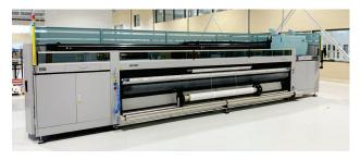
Instead of a traditional spray paint process, Annexair uses a super-wide digital printer to color our industrial Polyester film. With this machine, we have almost no limitations on printing possibilities.
