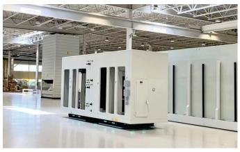
Each unit is assembled on one of our 40 Automated Guided Vehicule, following a path inside the factory
