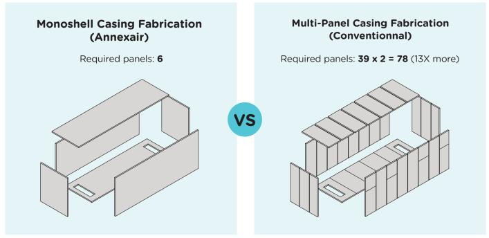
The illustration above shows the difference between Annexair biocomposite monoshell fabrication versus traditional multi-panel fabrication for a typical standard unit. As shown, the left image required less panels by a ratio of 1:13 versus the image on the right.
