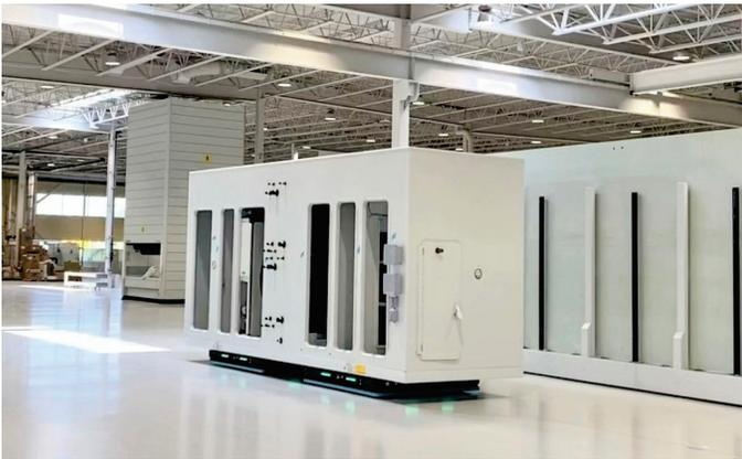
Each unit is assembled on one of our 40 Automated Guided Vehicle, following a path inside the factory
