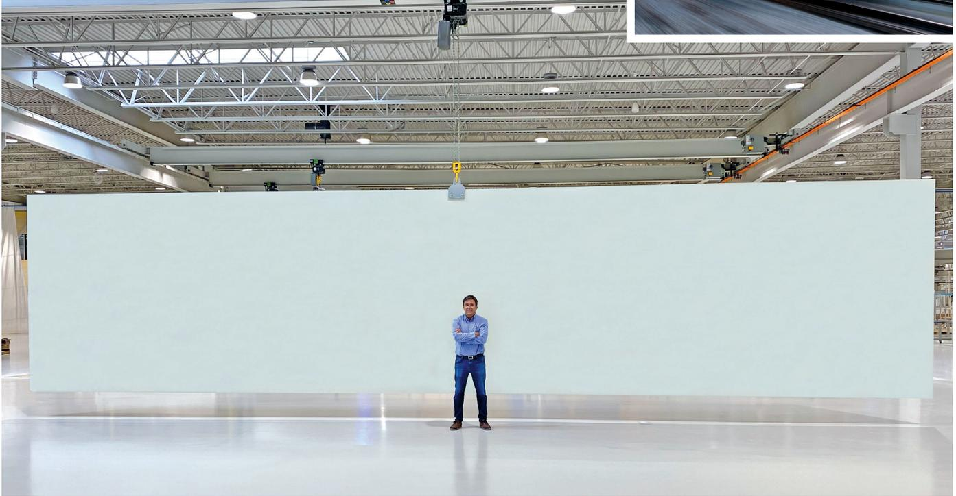
12 x 45 ft biocomposite panel made from 16,000 recycled plastic bottles
